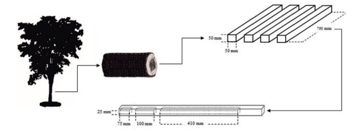
Figure 1. Schematic representation of a sample cutting for physical and mechanical tests of *Myracrodruon urundeuva* wood.
