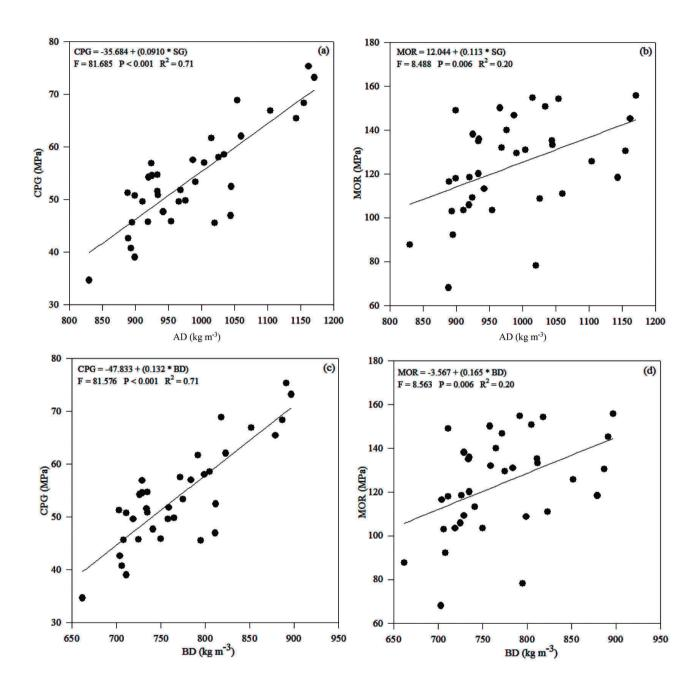
Figure 2. Relationships among properties of *Myracrodruon urundeuva* wood. a) Compression parallel to grain (CPG) as a function of apparent density (AD). b) Modulus of rupture (MOR) as a function of apparent density (AD). c) Compression parallel to grain (CPG) as a function of basic density (BD). d) Modulus of rupture (MOR) as a function of basic density (BD).
