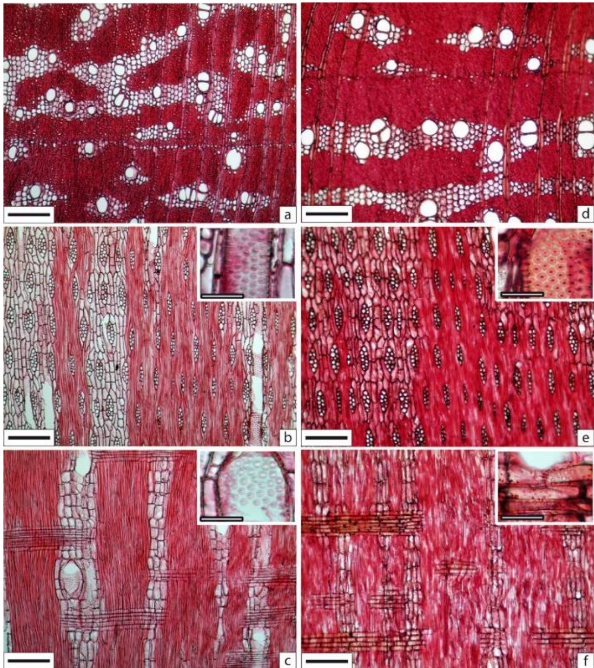
Figure 8. Wood sections of Handroanthus heptaphyllus (a, b, c), Handroanthus chrysotrichus (d, e, f), transversal sections (a, d) tangential sections with detail of the intervessel pits (b, e), radial sections with detail of the vessel-ray pits (c, f) Bar = 200 µm, detail bar = 50 µm.
